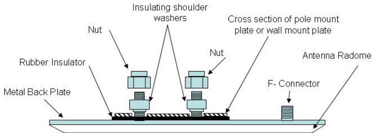
**Figure 8: Electrical Isolation of Antenna from Mount**
