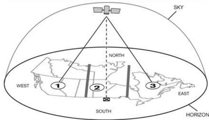
**Figure 10: SIRIUS Antenna Pointing Guidelines, Canada**
