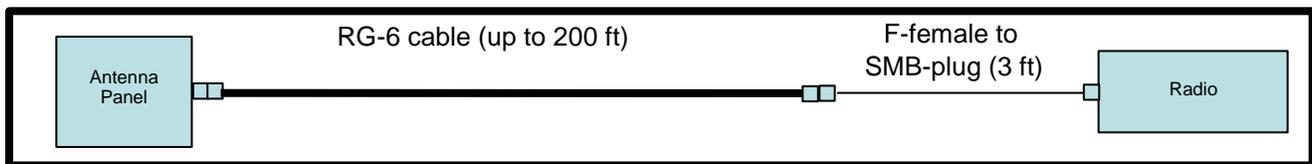
**Figure 5: Electrical Connections**
